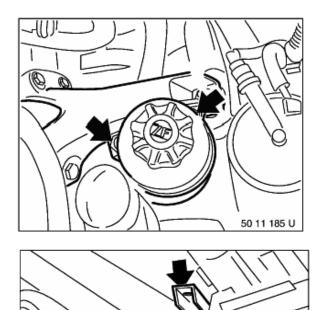
Drain power steering supply tank and tie back to one side (lines remain connected).
