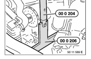
Carefully lift engine approx. 5 mm.
