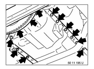
Unfasten oil pan screws at transmission and engine ends. Lower oil pan and pull forwards to remove.
