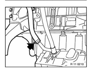
Remove oil return hose from cyclone oil separator on guide tube for oil dipstick.
